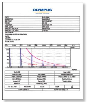
The EPOCH XT also offers onboard report generation. Operators may set up custom report headers and print directly from the instrument using the USB Host Port.
